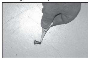
11. Apply the supplied loctite to the threads of the three supplied stand-off bolts as shown.
