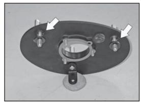
16. Install the factory breather bolts through the K&N back plate. On 2006 and later model year fuel injection models and all carbureted models, install the provided thick spacers (06403) onto the breather bolts as shown.
