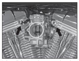
14. Install the breather extensions into the stock breather bolt location as shown.
