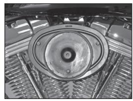
20. Install the K&N Air Filter and secure with the three bolts provided.
