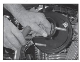
19. Tighten the three bolts that secure the back plate to the throttle body/carburetor. Then tighten the two breather bolts fully.
