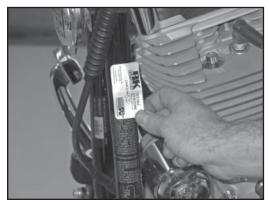
22. Install the E.O. sticker near the vehicle emissions label as shown.
