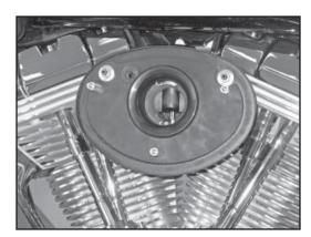
18. Install the back plate and secure with the stock breather bolts.
