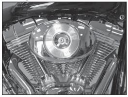
21. Reinstall the factory chrome cover and secure with the factory bolt.
