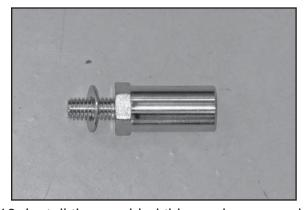
13. Install the provided thin washer on each of the two provided breather extensions as shown.
