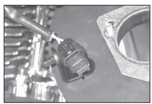
17. On vehicles equipped with an intake valve solenoid, install the intake valve solenoid connector into the bracket installed onto the rear of the backing plate. Secure with the provided tie wrap.
