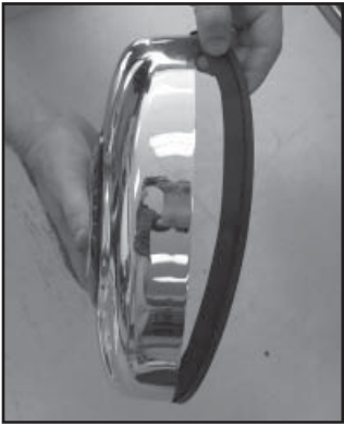
21. Remove the rubber trim from the stock air cleaner cover.
