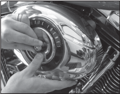
22. Reinstall the stock air cleaner cover and snugly tighten. Do not over-tighten.
