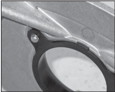
11. There should only be a few threads showing on the back of the back plate.
