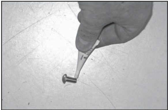
12. Apply Loctite to the threads of three of the button head socket bolts (item G on the parts list).
