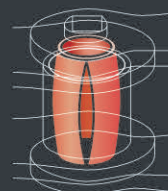
Curled bushing of a standard roller chain
